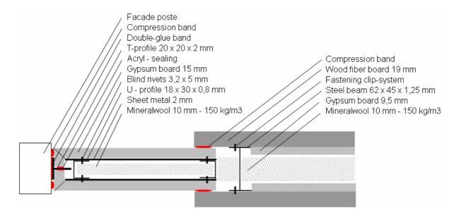
Measurements taken at the partition wall shown here of the sound reduction R'w demonstrate the influence of leaks, in this case in the area of the facade post.
