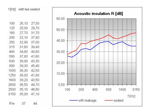
Where high acoustic reduction performance is required, a special attention must be paid to accidental leakages. The higher the performance of the wall, the more devastating are the negative influences of tiny acoustic by-passes (parasitic transmissions).
